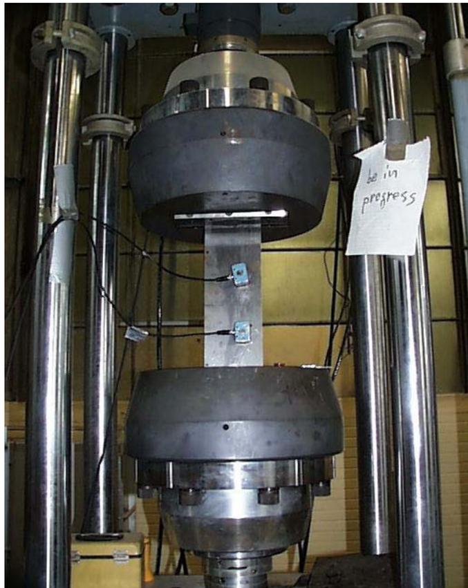
Figure 5.2 Overall View of AE Monitoring of Fatigue Crack Growth (1)
