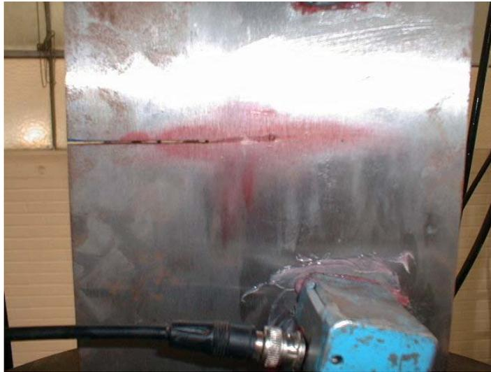
Figure 5.9 Fatigue Crack
