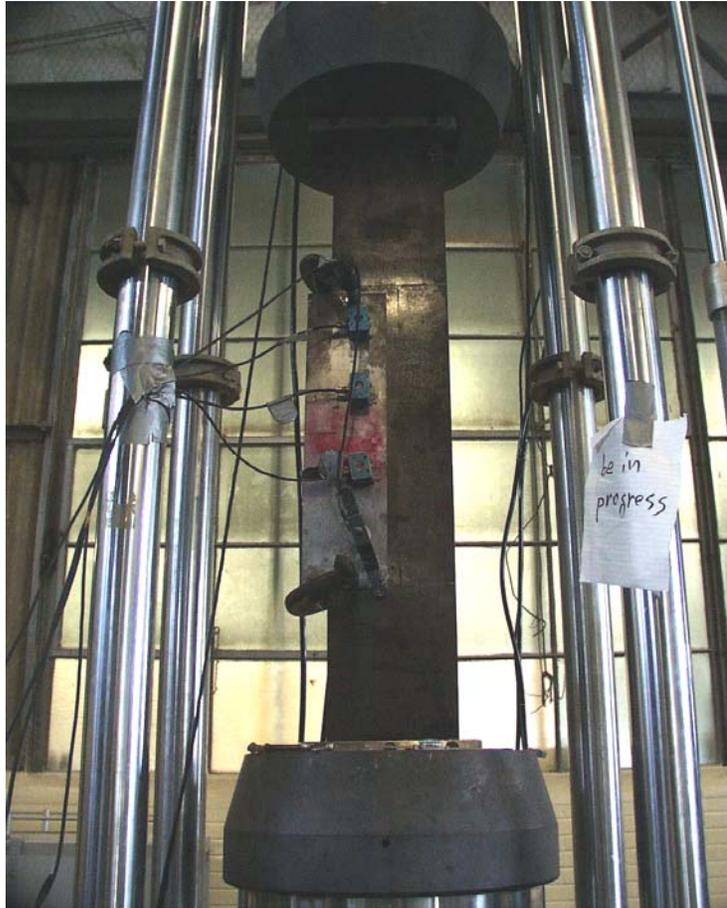
Figure 5.6 Overall View of AE Monitoring of Fatigue Crack Growth (2)
